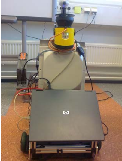
Figure 3. Mobile robot with RFID and safety scanner equipment.
