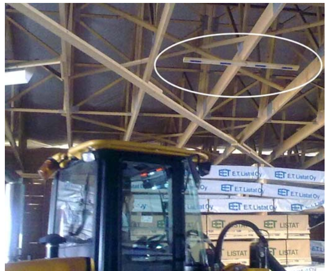
Figure 9. RFID tags in the ceiling used for indoor positioning.
