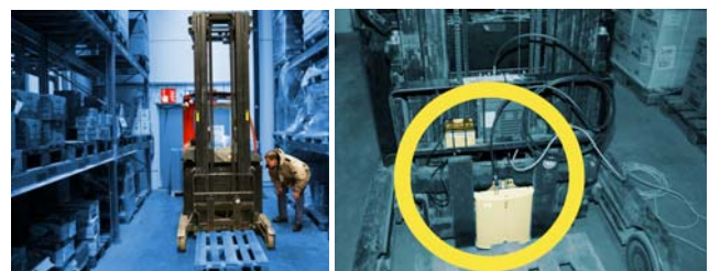
Figure 2. RFID equipped forklift truck in warehouse.
